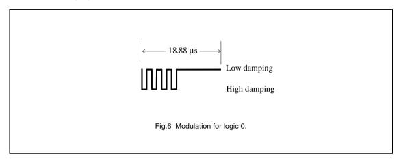
The waveforms in Figure 6, and similar diagrams to follow, represent logic states illustrating the periods of high damping and low damping of the antenna tuned circuit. They are not amplitudes of signals, but high oscillation amplitude will in fact occur during the high parts of the waveforms.
