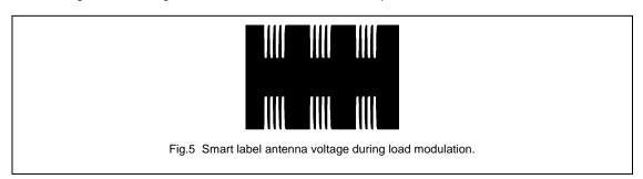
In the following description the physical state "modulator on" is named "high damping" and the physical state "modulator off" is named "low damping".
