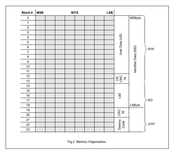
The I•CODE UID Smart Label IC memory contains, as shown in Figure 2, following elements:
