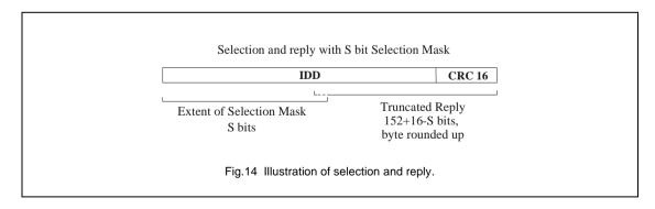
The Truncated Reply starts with the MSB at the preceding byte border of the truncated IDD and stops with the LSB of the CRC 16.
