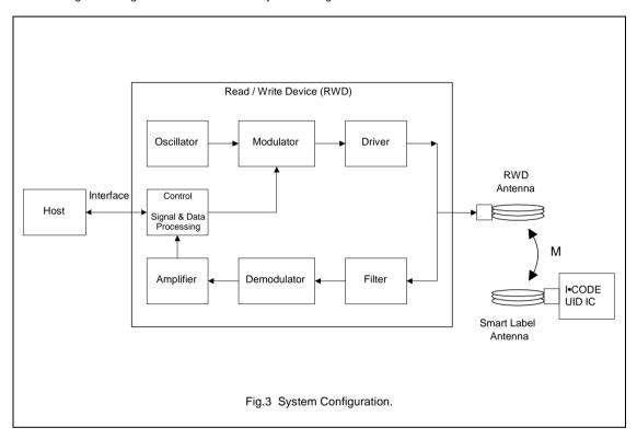
A control and data processing unit controls the modulation of the carrier signal and processes data coming back from the demodulator circuit.
